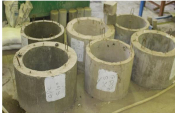
Fig. 6 Curing of pipes in ambient air
