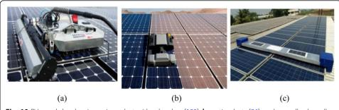
**Fig. 10** PV panel dry cleaning using robot with **a** brushes [103], **b** suction bots [26], and **c** small solar cells for charging its batteries and self-running [104]
