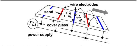
**Fig. 11** Schematic diagram of the electrostatic cleaning system that uses a standing wave and gravity to remove sand from a solar panel [109]
