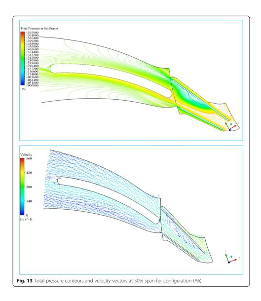
from the volute. This small difference in the pressure overcomes the formation of vortices and leads to improve the flow in diffuser-2. As a result, the static pressure recovery coefficient ( $C_{\rm pr}$ ) for the whole stage is increased by about 4:13%, as shown in Fig. 10, and the stage efficiency and pressure ratio are increased by about 0.17% and 0.2%, respectively, compared to configuration (A0).
