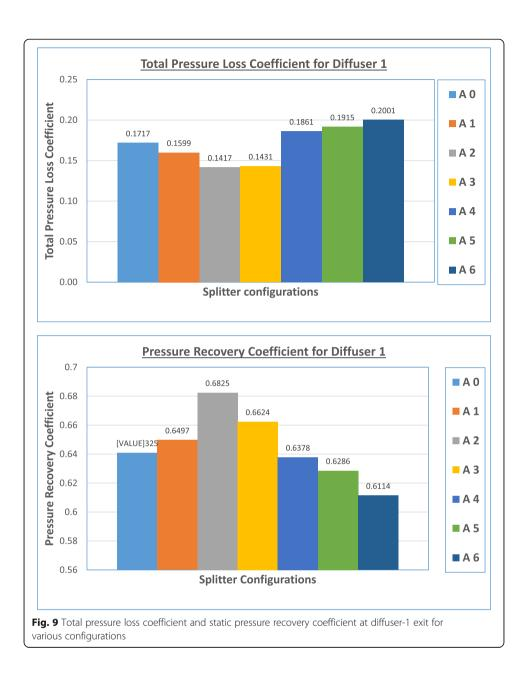
According to CFX calculations, the pressure recovery factor for diffuser-1 is 0.641, while the design area ratio predicts a  $C_{\rm pr}$  value of 0.721. The basic reason for this discrepancy is flow separation. This occurs when the boundary layers on the walls break away and cause an unfavorable reduction in performance. This break-away is also referred to as a stall that creates backflow in the diffusing region.
