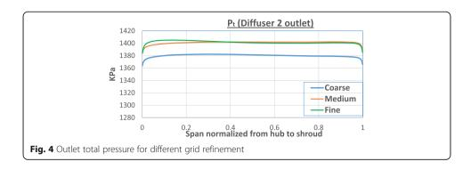
of interest into small sub-regions, called control volumes. The working fluid is air, with a molar mass equal of 28.96 kg/kmol. The thermodynamic properties have been obtained with the ideal gas equation of state, and with a four-coefficient zero-pressure polynomial equation for the specific heat capacity.
