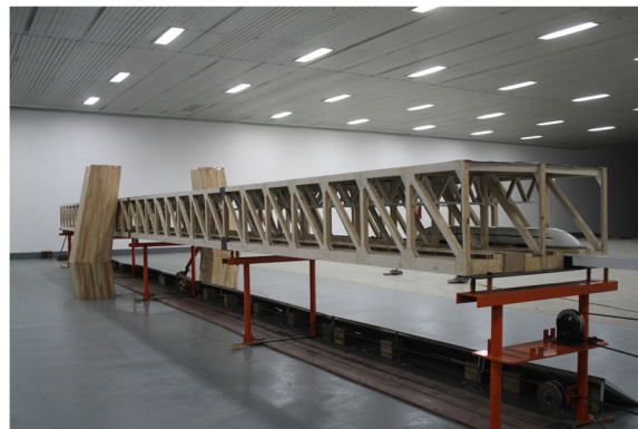
Fig. 21 Wind tunnel test of tower shielding on the aerodynamic characteristics of moving train (Li et al. 2019l)
