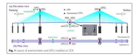
are included for action and response monitoring. This study will focus on the structural displacements and their dependencies with environmental factors including wind and temperature; sensors including anemometers, thermometers, and GPSs will be introduced briefly. Figure 1 exhibits the layout of anemometers and GPSs installed on SCB.
