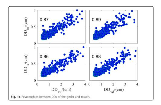
reason may be that the stayed cables connect the towers and the main girder and make them work together.
