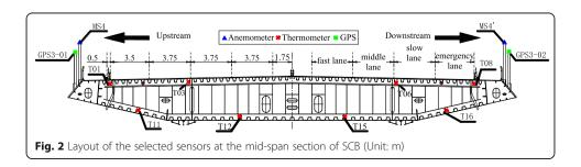
thermometers (T01, T03, T06, T08, T11, T12, T15, and T16) are selected to monitor and analyze the structural thermal distribution. As shown in Fig. 2, the selected eight thermometers are uniformly distributed around the mid-span section of the main girder. The sampling frequency of thermometers are 10 Hz.
