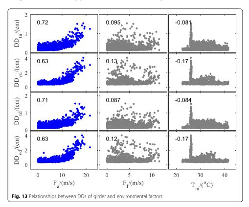
between DDs and longitudinal wind speed  $F_l$  is weak. Similarly, no obvious relationship can be found between DDs and structural temperature. During typhoon Haikui, the environmental temperature is concentrated around  $26\,^{\circ}$ C. The vibration amplitude increased to a high level during that time. Therefore, an obvious peak can be observed in the figure depicting correlation between temperature and vibration amplitude.
