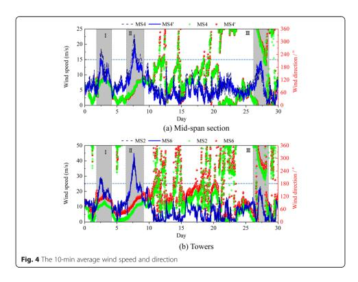
differences can still be identified during typhoon periods. As shown in Fig. 4(b), the measured wind speeds at two towers are almost the same, while constant differences between their direction angles can be observed. To minimize the influence of the bridge and its affiliations on the anemometers, the wind speed and direction measured at the inflow side of the bridge will be utilized for the following analysis.
