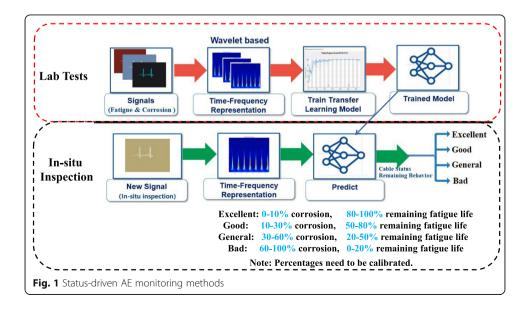
over-complete representation of the acoustic emission signals by translating and scaling parameter of the wavelets vary continuously, is employed to decompose the signals into frequency bands, and then achieve local time information via correlated resolution. Given a time series f(t), the continuous wavelet transform is expressed by the following integral:
