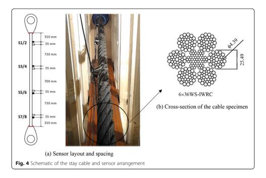
35 °C to 75 °C. Contact between sensors and cables was guaranteed by using couplant and insulation tape. The detection threshold is fixed at 35 dB for all sensors.
