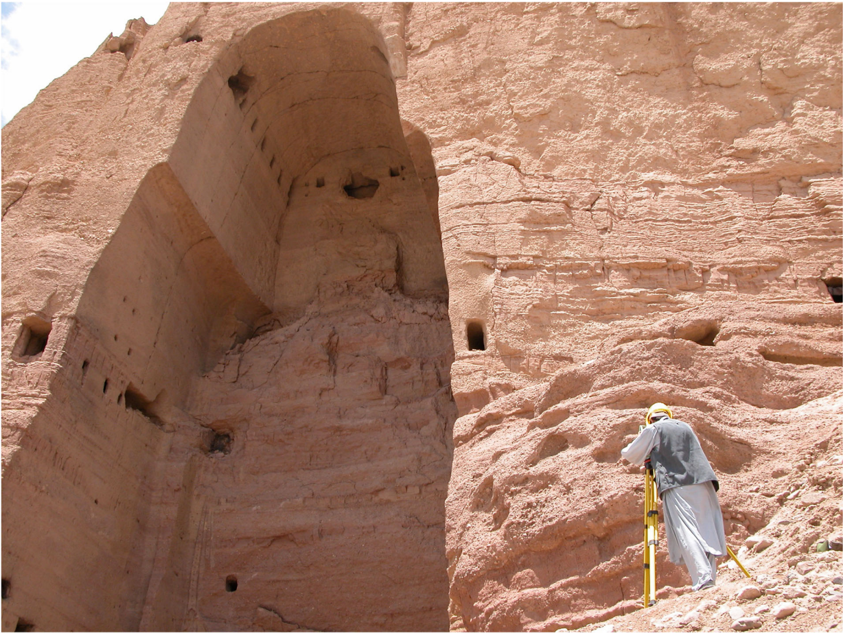
Fig. 6 Using a Total Station to record the deterioration of the Bamiyan Valley (2003) (Source: the authors)
