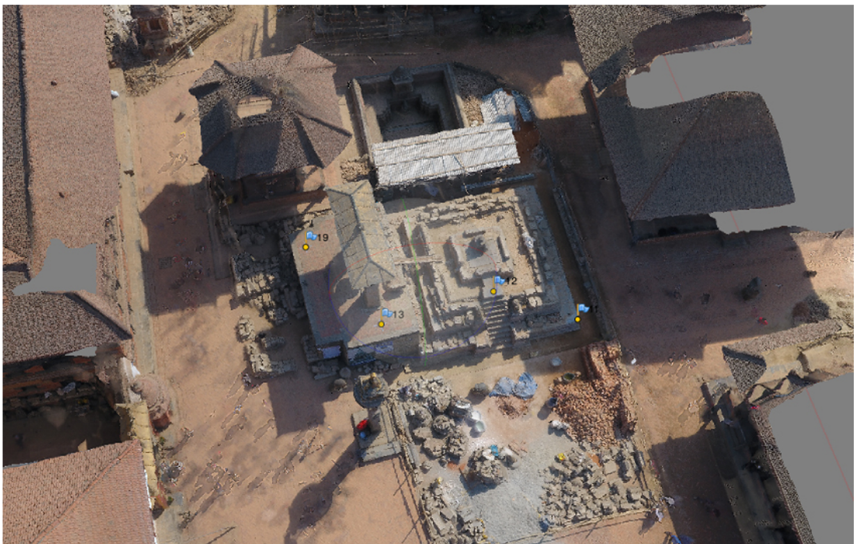
Fig. 8 Ortho-corrected image from aerial photogrammetry of the Bhaktapur Durbar Square after the earthquake (2017) (Source: the authors)
