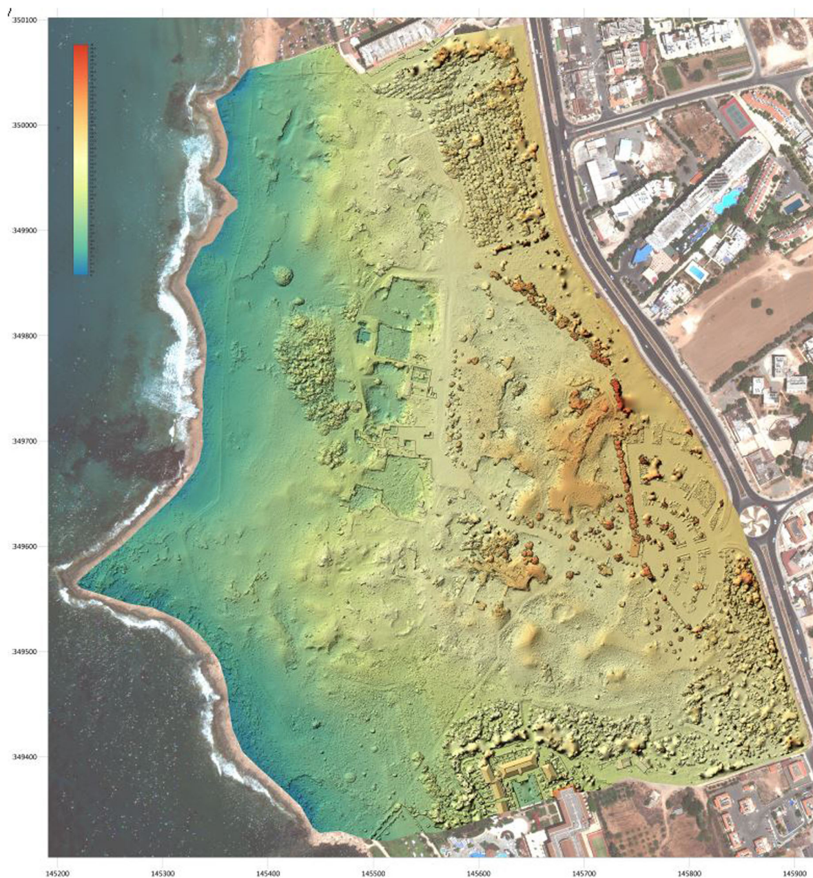
Fig. 16 Digital terrain model of one of the property's components (Source: the authors)
