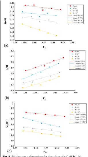
**Fig. 3** Relative scour dimensions for the values of **a**  $D_s/H$ ; **b**  $L_s/H$ ; and **c**  $V_s/H^3$  versus  $F_{r1}$  for the tested flow jet arrangements at gate opening G=6 cm
