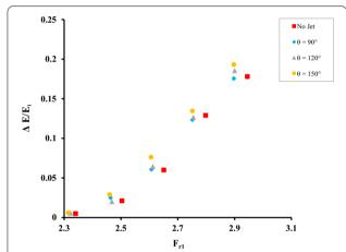
**Fig. 2** Relative energy dissipation  $\Delta E/E_1$  versus  $F_{r_1}$  for the tested flow jet arrangements at gate opening G = 7 cm
