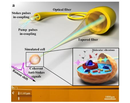
**Fig.1** Principle of a CARS tapered optical fiber probes for single-cell minimally invasive endoscopy. **a** Illustration and **(b)** photography of fabricated device including a tapered fiber tip. **c** Enlarged view of the fiber tip
