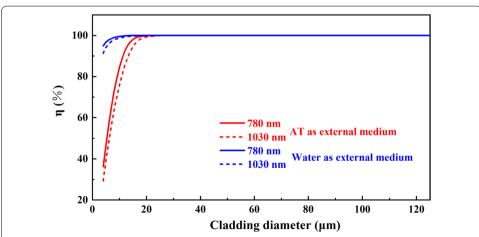
**Fig.4** The calculated results of the fraction of optical power in the fiber  $\eta$  with 4  $\mu$ m to 125  $\mu$ m cladding diameters. The blue line denotes that the external medium is water, and the red line denotes that the external medium is ATs. The  $\eta$  is 92.4% at 780 nm and 85.3% at 1030 nm when the cladding diameter is 12  $\mu$ m and the external medium is ATs
