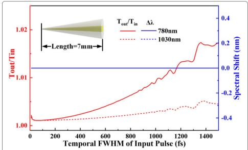
**Fig.6** The calculated time domain broadening and the spectral shift of ultrashort pulses with different pulse widths transmitted by a 7 mm tapered optical fiber probe. The total time domain broadening ratio is < 1.02 for 780 nm pulses and < 1.005 for 1030 nm pulses
