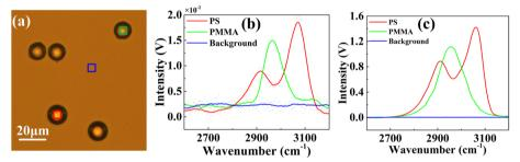
**Fig.7** a Microscope image of PS microsphere and PMMA microsphere samples, the blue, red and green squares represent the slide background, PS microsphere, and PMMA microsphere, respectively. **b** CARS signals detected by the optical fiber probe and **c** free-space elements. The blue, red and green solid lines represent the signals of slide background, PS microsphere, and PMMA microsphere, respectively
