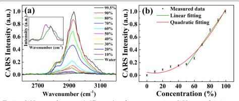
**Fig.10 a** CARS spectra of acetone with different volume fractions in water. Inset: CARS spectra of 10 v/v% acetone and water. **b** Relative CARS intensity at  $2921 \text{ cm}^{-1}$  for increasing volume fractions of acetone in water.
