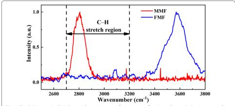
**Fig.3** The FWM signals of MMF cover from ~2700 cm<sup>-1</sup> to 2900 cm<sup>-1</sup> and interfere with the detection of C–H bond vibrations. The FWM signals of FMF cover from ~3400 cm<sup>-1</sup> to 3800 cm<sup>-1</sup> and avoid interference to the detection of C–H bond vibrations
