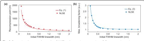
**Fig. 3** Comparison between the results of NLSE and approximate equations. **A** Recompression point as a function of initial FWHM linewidth. **B** Maximum RMS-BF dependence on the initial FWHM linewidth. Lines: solutions of the approximate equations. Scatters: simulated results based on NLSE
