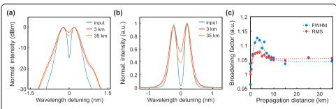
**Fig. 6** Experimental spectral evolutions of double-peak spectra. **A** Output spectra in logarithmic scale at 3 different positions: input, 3 and 35 km. It's worth noting that the spectral FWHM linewidth broadens to its maximum with 3-km propagation. **B** Output spectra in linear scale. **C** Spectral broadening factors dependence on the propagation distance. Scatters: experimental data; lines: spline fitting
