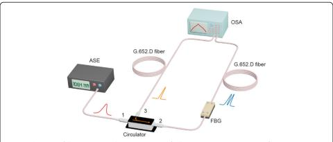
**Fig. 4** Schematic of the experimental setup. ASE, amplified spontaneous emission; FBG, fiber Bragg grating; OSA, optical spectrum analyzer
