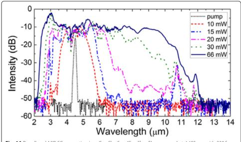
**Fig. 16** Broadband MIR SC generation in a  $Ge_{15}Sb_{15}Se_{70}/Ge_{20}Sb_{80}$  fiber pumped at 4.485  $\mu$ m with 330 fs pulses (Adapted with permission from [89], copyright John Wiley & Sons)
