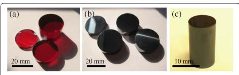
**Fig. 1** Three typical ChG glasses. **a**  $As_2S_3$ . **b**  $As_2Se_3$ . **c**  $Ge_{20}As_{20}Se_{15}Te_{45}$  (Adapted with permission from [36], copyright SPIE)
