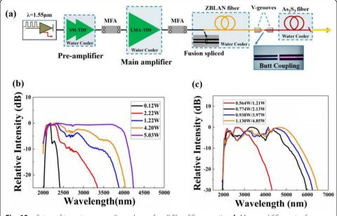
**Fig. 12 a** Setup of two-stage cascading scheme for all-fiber SC generation. **b** Measured SC spectra from ZBLAN with different output powers. **c** Measured SC spectra from  $As_2S_3$  fiber with different output power versus the input power (Adapted with permission from [29], copyright the Optical Society)
