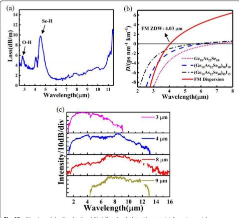
**Fig. 19 a** Fiber loss of the  $Ge_{10}As_{22}Se_{68}$ -I ChH fiber. **b** calculated the material dispersion and the fundamental mode dispersion curves of the  $Ge_{10}As_{22}Se_{68}$ -I ChH fiber. **c** SC spectra from the  $Ge_{10}As_{22}Se_{68}$ -I ChH fiber pumped with different wavelengths (Adapted with permission from [97], copyright the Optical Society)
