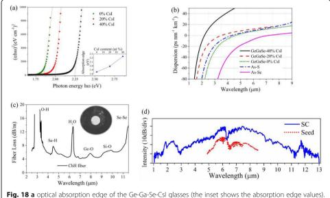
**Fig. 18 a** optical absorption edge of the Ge-Ga-Se-CsI glasses (the inset shows the absorption edge values). **b** Calculated material dispersion of ChH glasses. **c** optical loss of the ChH fiber. **d** SC generation in the ChH fiber pumped at 6.3 µm (Adapted with permission from [96], copyright John Wiley & Sons)
