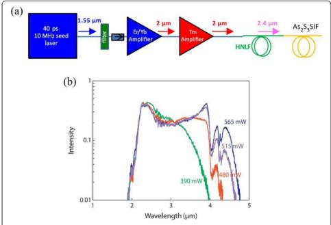
**Fig. 6 a** A typical schematic of SC generation based on a MOPA pump system. **b** SC generation in a 2-m-long step-index As<sub>2</sub>S<sub>3</sub> fiber with a wide spectral coverage of 1.9–4.8 μm and a high average output power of 565 mW (Adapted with permission from [60], copyright Elsevier B. V)
