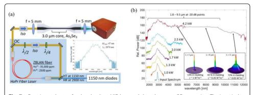
**Fig. 7 a** Experimental setup for the ultrashort MIR laser and the subsequent SC generation. The inset is the optical spectrum of the pump pulses. **b** SC generation in the As<sub>2</sub>Se<sub>3</sub> TF pumped by increasing peak power (Adapted with permission from [70], copyright the Optical Society)
