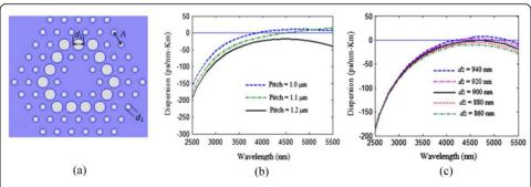
**Fig. 4 a** Cross-section of a triangular-core MOF. Dispersion curves as a function of wavelength varying **b** the pitch and **c** the air hole diameter (Adapted with permission from [22], copyright Elsevier B. V)
