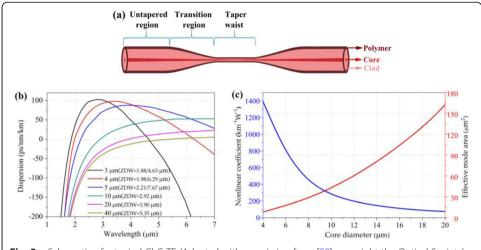
**Fig. 3 a** Schematic of a typical ChG TF (Adapted with permission from [50], copyright the Optical Society). **b** Dispersion, **c** Nonlinear coefficient and effective mode area of a ChG TF with As<sub>2</sub>Se<sub>3</sub> core and As<sub>2</sub>S<sub>3</sub> cladding as a function of the fiber core diameter
