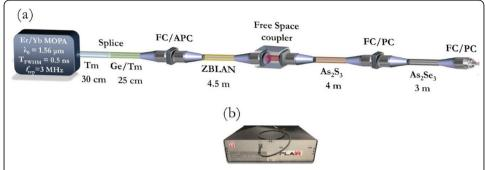
**Fig. 14 a** Setup of three-stage cascading SC source without thulium amplifier. **b** Packaged SC source. **c** Measured SC spectra from ZBLAN (blue), As<sub>2</sub>S<sub>3</sub> (red), and As<sub>2</sub>Se<sub>3</sub> (black) fibers (Adapted with permission from [79], copyright the Optical Society)
