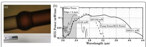
**Fig. 8 a** Micrograph of the fusion splice between silica and ChG fibers. **b** SC generation in the  $As_2S_3$  fiber pumped by pulsed laser at 2.5  $\mu$ m (Adapted with permission from [71], copyright the Optical Society)
