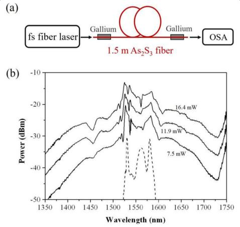
**Fig. 5 a** Experimental setup for SC generation in an  $As_2S_3$  step-index fiber pumped by a Er-doped fiber laser. **b** SC sources generated from an  $As_2S_3$  step-index fiber (Adapted with permission from [59], copyright the Optical Society)
