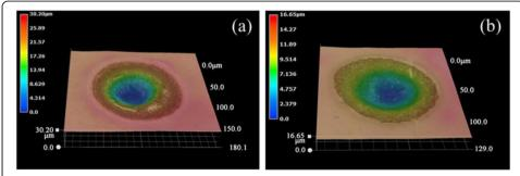
**Fig. 15** Optical microscope images of laser-induced damage sites after irradiation with a 3  $\mu$ m fs laser at 30 mW and 20 s duration. **a** As<sub>2</sub>Se<sub>3</sub> glass; **b** Ge<sub>15</sub>Sb<sub>25</sub>Se<sub>60</sub> glass (Adapted with permission from [88], copyright the Optical Society)
