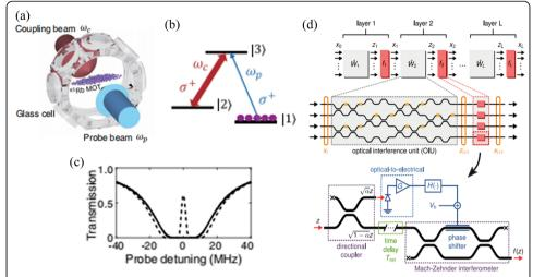
**Fig. 10 a**, **b**, **c** represents the preparation, energy level diagram, and transmission diagram of laser-cooled <sup>85</sup>*Rb* atom, respectively [34, 82]. **d** An electro-optical nonlinear activation function structure can be used to realize the optical nonlinear element ONU [83]
