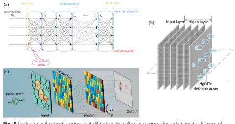
**Fig. 3** Optical neural networks using light diffraction to realize linear operation. **a** Schematic diagram of deep diffraction neural network D<sup>2</sup>NN [24]. **b** Diffraction grating network system [25]. **c** Metasurface implements optical logical operations [26]
