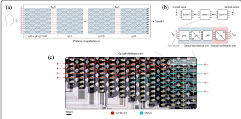
**Fig. 5** Using the principle of interference to realize the linear operation in the neural network [36]. **a** Coherent nanophotonic circuit. **b** Each layer of the neural network is composed of optical interference unit OIU and optical nonlinear unit ONU. **c** The internal structure of OIU unit
