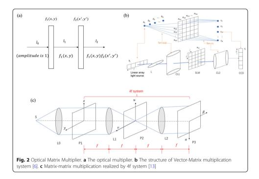
The optical matrix multiplier fully embodies the parallel computing power of light, and the optical linear operation completed by OMM is essentially to realize the modulation of information-carrying light by means of certain approaches and some properties of light, such as diffraction, interference and so on.
