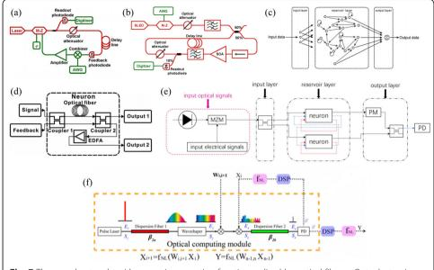
**Fig. 7** The neural networks with reservoir computing function realized by optical fiber. **a** Optoelectronic reservoir computing [51]. **b** All-optical reservoir computing [52]. **c**, **d**, **e** respectively describes the principle of reservoir computing, and the structures of the neuron and neural network constructed based on the optical fiber communication system [53]. **f** A serial electro-optic neural network based on time-domain stretching [54]
