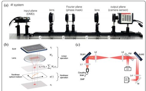
**Fig. 4** Optical neural networks with linear operation realized by Fourier transform of light [33]. **a** Optical convolution operation is realized by 4f system. **b** Experimental realization of optical neurons in AONN [34]. **c** The linear operating system of AONN [34]
