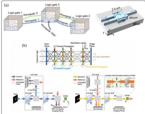
Fig. 11 a Possible solutions for optical logic gate cascading and other possible implementation platforms [26]. b Describes a SLM cascade neural network, and uses 4f system and SLM to realize optical field measurement, thereby carrying out optical training of diffraction ONN [85]
