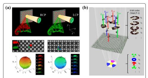
**Fig. 2** Color holography based on metasurfaces. **a** Illustration of the polarization-controlled color hologram. The color of the reconstructed images can be tuned by changing the polarization of incident light [67]. **b** Schematic illustrations of the transmitted 6-bit metasurface consists of silicon nanobricks arrays with spatially varying orientations on a quartz substrate [65]
