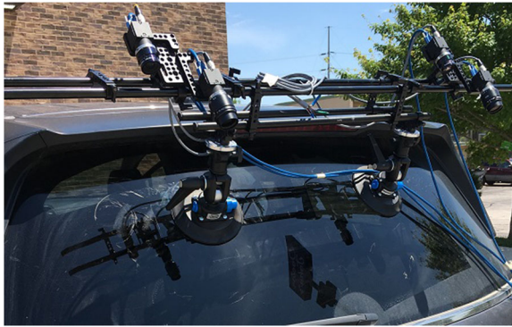
Fig. 3 High-resolution images collected from machine-vision cameras mounted on a vehicle
