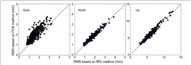
**Fig. 7** RMS of the transformed position residuals based on the alternative IRC method against those based on the FCBs for each day over 1 year. Note that the scale for the Up component differs from those for the horizontal components
