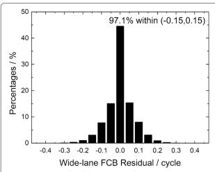
**Fig. 3** Distribution of the fractional parts of all the FCB-corrected wide-lane SD-ambiguities. Black is the result from the network of all stations, where approximately 97.1% are close to an integer within 0.15 cycles
