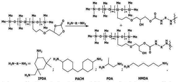
Fig. 5 Synthetic routes of the NIPU coatings.based on cyclic Polysiloxanes [63]. Copyright 2017, The Author(s), under the terms of the Creative Commons CC BY license
