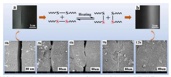
Fig. 2 Self-healing process of leather coating: a damaged leather coating; b leather coating after be repaired at 60 °C for 12 h. SEM images show the self-healing process in time. Copyright 2020, The Author(s), under the terms of the Creative Commons CC BY license [60]
