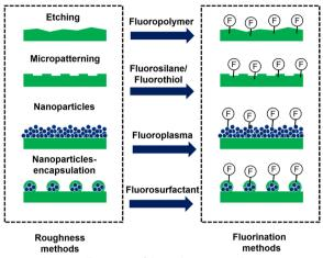
**Fig. 3** Schematic illustration of the techniques used to create superhydrophobic surfaces
