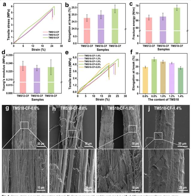
Fig. 6 Stress–strain curves (a), elongation at break (b), fracture energy (c), and Young's modulus (d) of different collagen fibers, stress–strain curves of TMS18-CF with different content of TMS18 (e), elongation at break of TMS18-CF with different content of TMS18 (f), SEM images of TMS18-CF-0.6% (g), TMS18-CF-0.8% (h), TMS18-CF-1.0% (i), TMS18-CF-1.4% (j)
