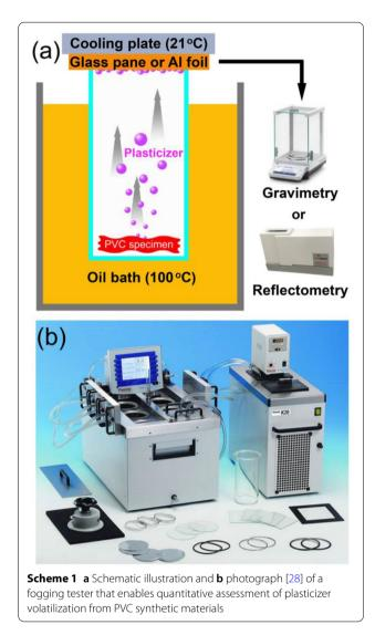
oil bath at 100 °C for 16 h, the foil is removed and dried over a desiccant for 4 h before re-weighing. The fogging value *G* is given by the difference between the masses of the aluminium foil after and before fogging. The results obtained from the reflectometric method and the gravimetric method are not directly related to each other as they measure different parameters.
