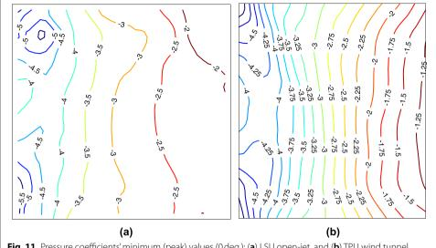
**Fig. 11** Pressure coefficients' minimum (peak) values (0 deg.): (a) LSU open-jet, and (b) TPU wind tunnel (wind from left to right)
