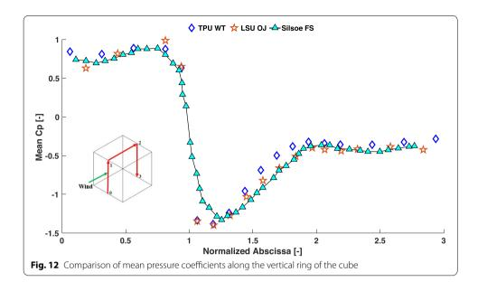
realization to another, which stems from the highly fluctuating nature of wind. In the experiment, the angle of incidence is normal to the windward face of the cube, which is considered as the 0-degree case in this paper.
