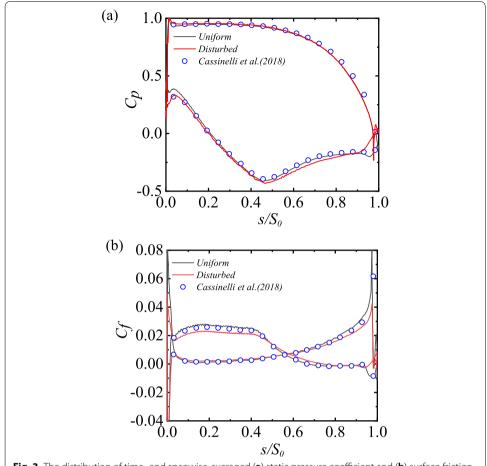
**Fig. 3** The distribution of time- and spanwise-averaged (a) static pressure coefficient and (b) surface friction coefficient
