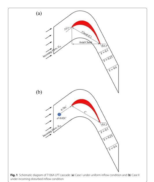
cascade as a wake-type disturbance in the case II. A moderate inflow Reynolds number of  $Re_{\infty} = 50,000$  (based on inflow velocity  $U_{\infty} = 1$  and chord C = 1) is employed, which corresponds approximately to  $Re_2 = 88,450$  (based on the mixed-out velocity magnitude at the exit measurement plane).
