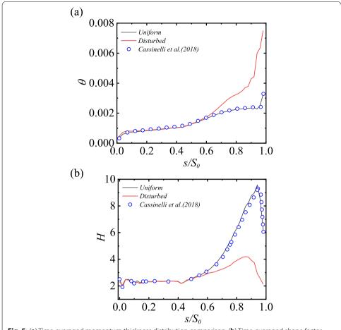
**Fig. 5** (a) Time-averaged momentum thickness distribution comparison; (b) Time-averaged shape factor comparison
