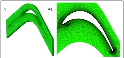
**Fig. 2** Mesh of disturbed case II: **(a)** macroscopic finite element grid distribution of computational domain and **(b)** zoomed in grid near the blade wall
