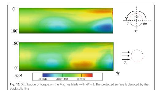
Further simulations of a spinning cylinder with differing aspect ratios were carried out to provide an insight on its influence on the Magnus effect. At the same Reynolds number of  $1.0 \times 10^5$  and velocity ratio of 2.0, the design with AR = 10 showed a decrease in observed lift coefficient. The observed aspect ratio dependency was evidenced by the three-dimensionality of the near-wake behind the spinning cylinder.
