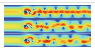
**Fig. 3** The flow patterns of the flow over a square cylinder at Re = 300. Top: MRT-LBE, mesh size  $2000 \times 320$ ; Middle: MRT-LBE, mesh size  $5000 \times 800$ ; Bottom: DUGKS, mesh size  $2000 \times 320$
