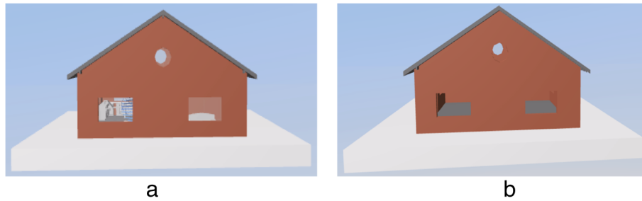
Fig. 2 External component extraction based on the bounding box. The external windows and doors are extracted incorrectly. a Original model b Result based on the bounding box algorithm
