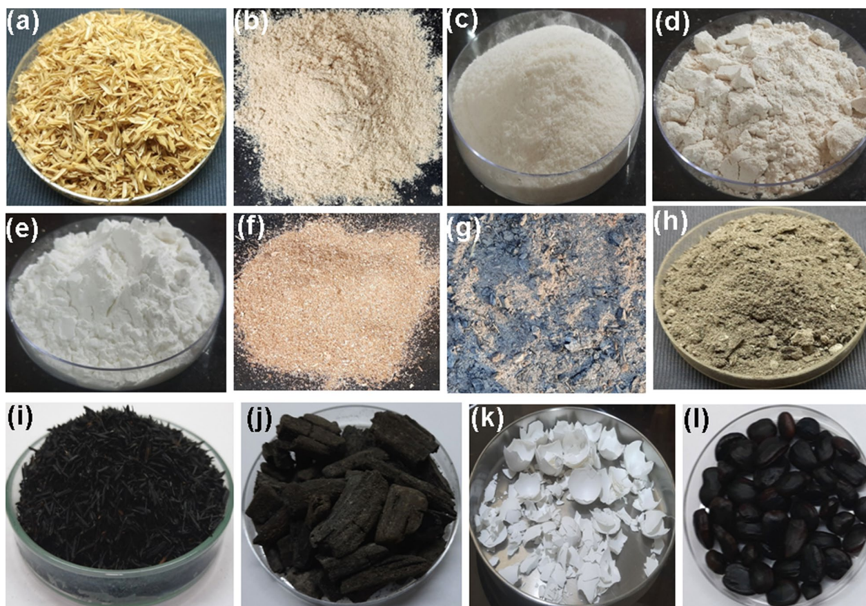
Fig. 4 Photographs of Indian traditional, natural abrasives used for dish wash cleaning, a rice husk, b rice bran, c rice starch, d wheat starch, e corn starch, f saw dust, g wood ash, h dung ash, i rice husk biochar, j charcoal, k egg shells and l tamarind seeds
