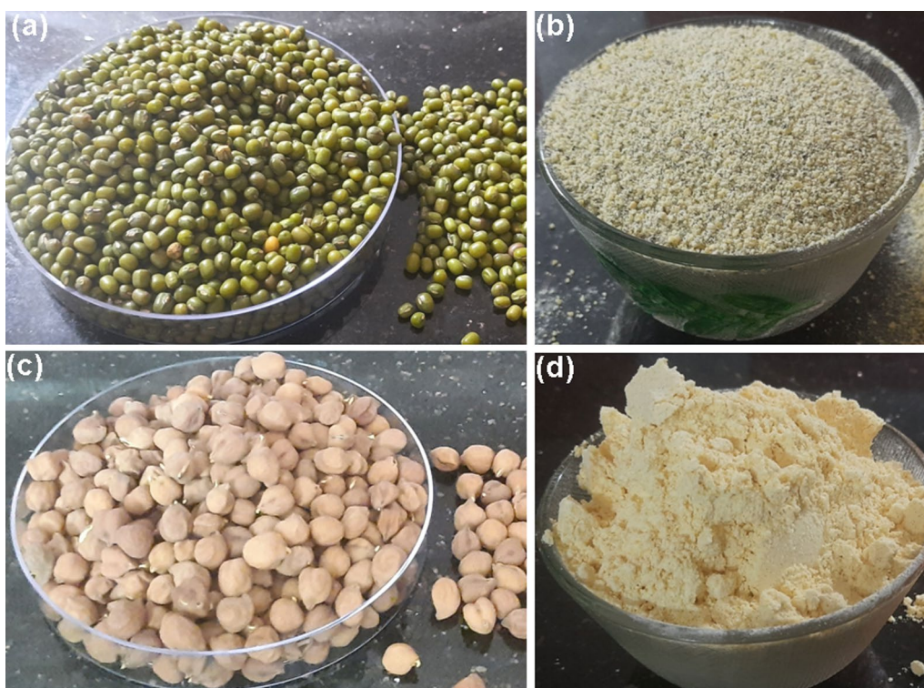
Fig. 9 Photographs of Indian traditional, natural saponin biosurfactants used for dish wash cleaning, a green gram seeds, b green gram seed powder, c Bengal gram seeds and d Bengal gram seed powder
