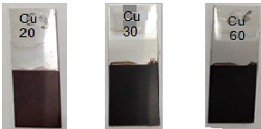
Fig. 2 Colored with Cu only using anodization time of 20, 30 and 60 min
