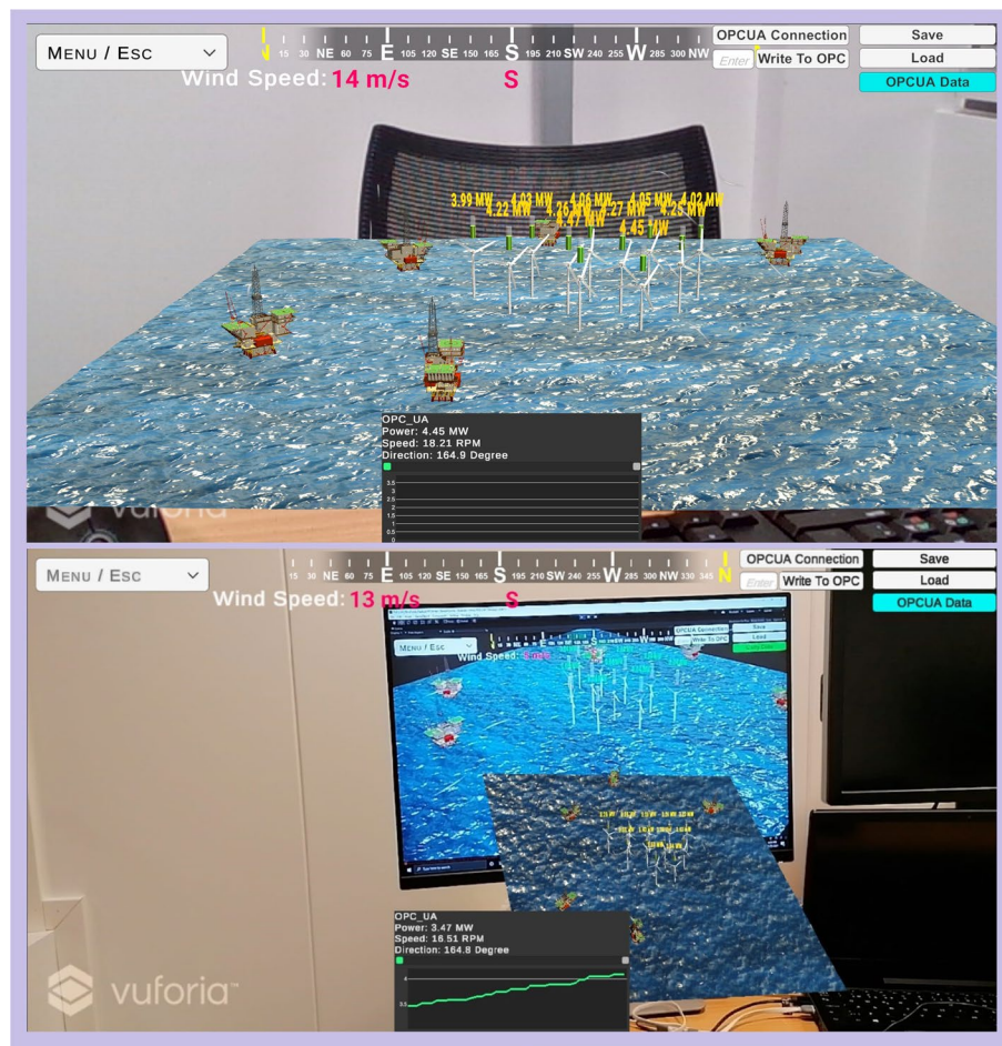
Fig. 14 The augmented reality-based visualization of a digital twin of a wind farm
