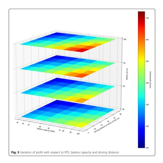
round trip efficiency, there is an increase of 1.62 Euros in profit. For every 1 kWh increase in battery capacity, the profit increases by 1.85 Euros. For every 1 km decrease in driving distance per trip, profit increases by 6.64 Euros. Fig. 6 summarizes the sensitivity of energy transferred per year with respect to the above parameters. For more details on the sensitivity analysis we refer to (Malya, 2020).
