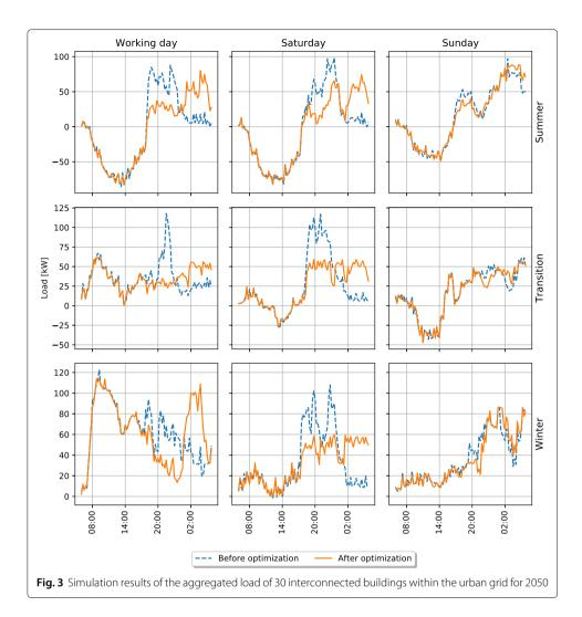
The reduction of the load peaks works differently well, depending on the type of the peak. Negative load peaks due to the feed-in of photovoltaic systems can hardly be reduced. The reason for that is that there is usually only little flexibility available during the period of feed-in within the smart buildings. Additionally, the existing flexibility is
