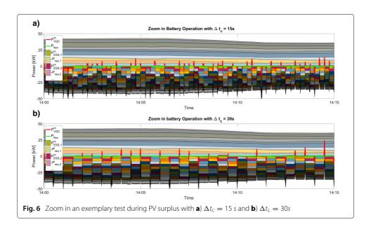
aggregated power at the virtual grid connection  $P_{VGC}^{m}$  is displayed in red. As no flexibility is contracted (green line), the set value for the virtual grid connection in zero.
