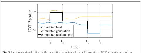
Fig. 3 Exemplary visualization of the operating principle of the self-organized DVPP (producer counting arrow system)
