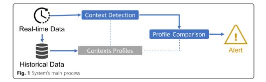
When comparing the instant consumption with the previously generated context profiles, it is important to aggregate the instant data in a higher level of granularity (e.g. last minute), which reduces its variable nature and therefore guarantees more solid data, avoiding misleading alarms.
