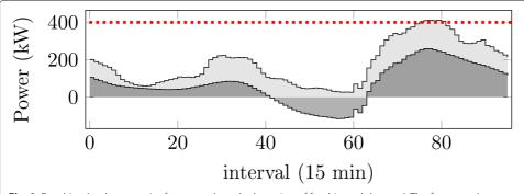
**Fig. 9** Resulting load prognosis after agent-based adaptation of feed-in and demand. The forecasted overload has been largely reduced. The darker area represents non-controllable loads
