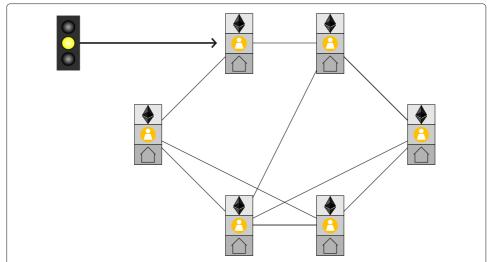
**Fig. 3** Overview on layered system architecture: Depending on a congestion warning (displayed as yellow traffic light), the agents cooperate using household simulation, cooperative agent layer and blockchain agent layer
