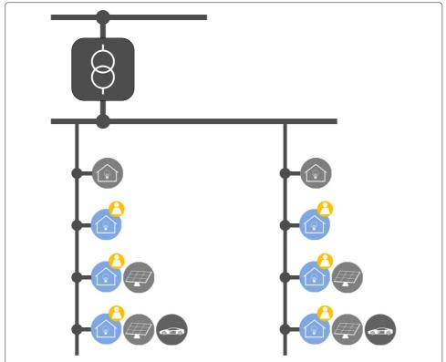
**Fig. 4** Showcase grid scenario: Non-controllable loads (grey houses) and controllable generation and load components (with agent symbol in yellow) connected to a transformer
