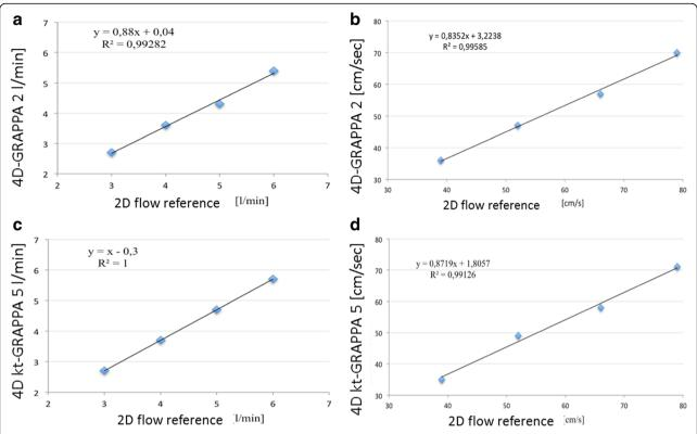
**Fig. 5** Scatter plots of the correlation between flow volumes and mean flow velocity measured with the 4D flow GRAPPA2 and *k-t*-GRAPPA5 sequences and the 2D flow sequence (reference) in pulsatile flow. **a, c** Flow volume [L/min]. **b, d** Mean flow velocity [cm/s]. 2D, two-dimensional; 4D, four-dimensional; cm/s, centimetres per second; GRAPPA, generalised autocalibrating partially parallel acquisition; L/min, litres per minute
