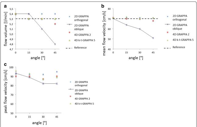
**Fig. 4** Influence of misalignment of the measuring plane on 2D flow and 4D flow measurements in constant flow regarding the (a) flow volume [L/min], (b) mean flow velocity [cm/s], and (c) peak flow velocity [cm/s]. 2D, two-dimensional; 4D, four-dimensional; cm/s, centimetres per second; GRAPPA, generalised autocalibrating partially parallel acquisition
