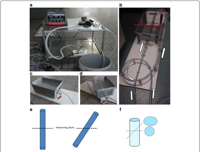
**Fig. 1 a, b** Overview of the blood pump with control panel and inflow and outflow tubes. **c, d** The plastic tub filled with carbopol gel containing the tissue tube could be rotated. The red arrow indicates a goniometer. **c** Orthogonal orientation. **d** 45° rotation. **e** Schematic showing 2D flow measurements with the phantom vessel positioned along the *z*-direction of the MRI scanner (0°) and with an altered angle (45°). **f** Schematic changes of the cross-sectional area and shape
