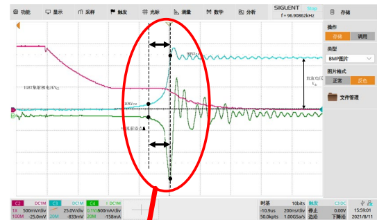
Fig. 13 The consistency of high-frequency pulse signal and voltage mutation during the turn-off process
