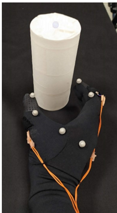
Fig. 2 Picture of the sensory substitution glove. Note. Picture of the sensory substitution glove. The device consists of a regular polyester glove with six reflective markers (white semispheres) and two vibrotactile coin motors (one on the index finger and one on the thumb) which were inside a pocket
