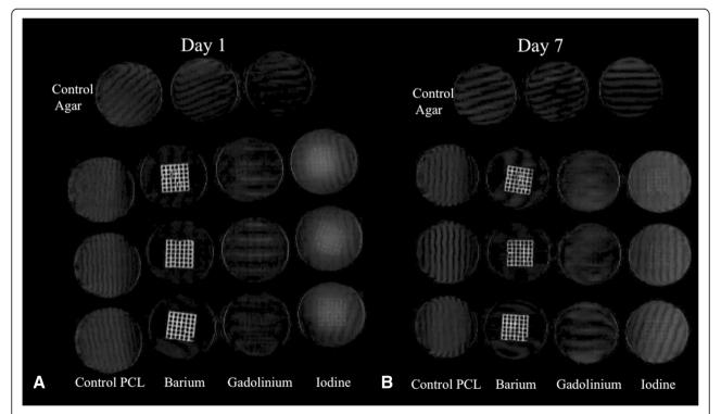
**Fig. 2** Coronal volume rendering of the contrast impregnated and control meshes in the 37 °C. agar solution at day 1 (**a**) and day 7 (**b**). Note the visibility of the barium mesh sustained at both time periods, poor perceptibility of the gadolinium meshes at either time period, and that more iodine is present in the surrounding agar at day 7 (**b**) compared to day 1 (**a**)
