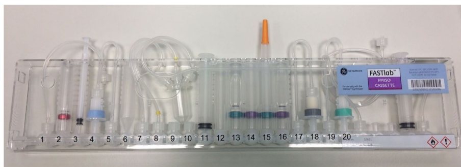
Fig. 4 FASTlab cassette for [ ^{18}\text{F} ]FMISO, for reagents see Table 2
