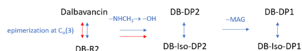
Fig. 10 Schematic comparison of the degradation pathways at 40 °C and 70 °C. Red arrows indicate the processes that are observed at 40 °C, and blue arrows indicate processes that are observed at 70 °C
