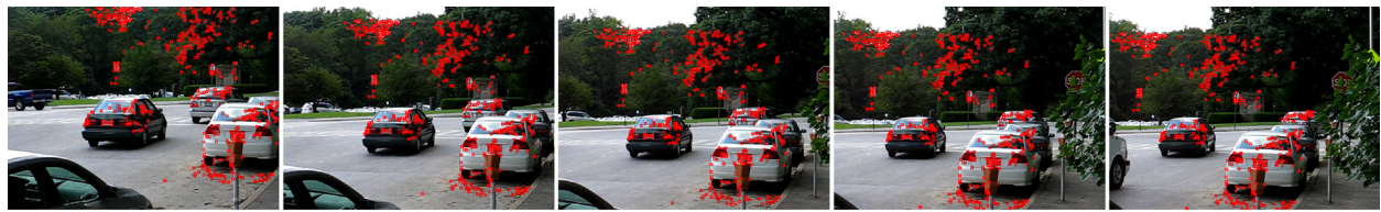
(a) The input video sequence of 30 frames, which are the first, 8th, 15th, 23th, and 30th frame respectively. Red points are the tracked feature points.
