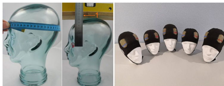
Fig. 3 Measurement of head circumference and distance between eye angle and vertex (1). Five cap sizes for different head shapes
