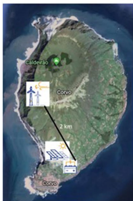
Figure 22.7: Corvo Island Hybrid System
