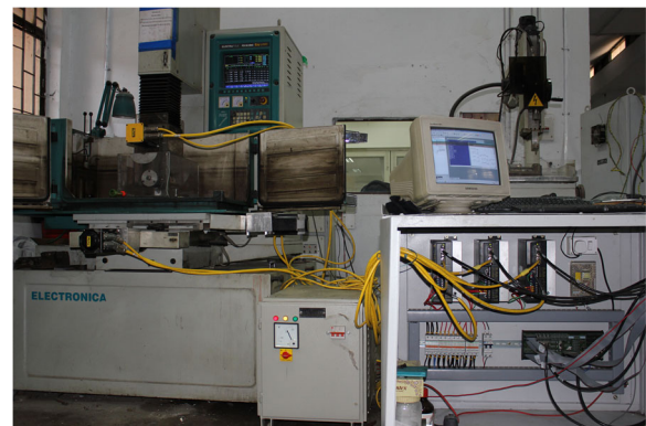
Fig. 2 Attached experimental setup on EDM machine
