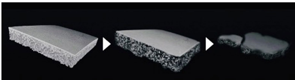
Fig. 7 Schematic images of poly (L-lactic acid) and poly (ε-caprolactone) (PLACL) degradation provided by GC, Tokyo, Japan
