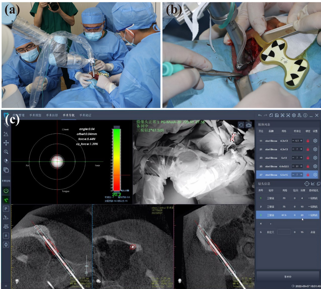
Fig. 8 Intraoperative image and autonomous site preparation procedure. The autonomous zygomatic implant site preparation was achieved by the image-guided robotic surgery system (a, b). Robot-assisted surgical software system provide real-time feedback of the robotic arm and the drill in surgery (c)
