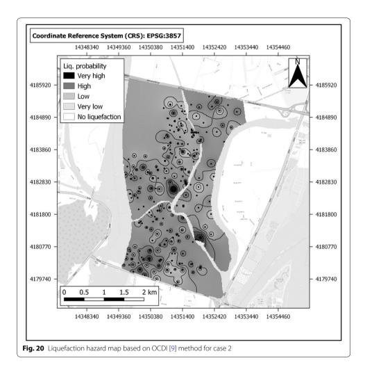
[9]. These figures show that the fines content have a significant effect on the liquefaction probability, since the severity of liquefaction dramatically changes from case 1 to case 2 and from case 2 to case 3. It is seen that the probability of liquefaction is almost low for case 3.
