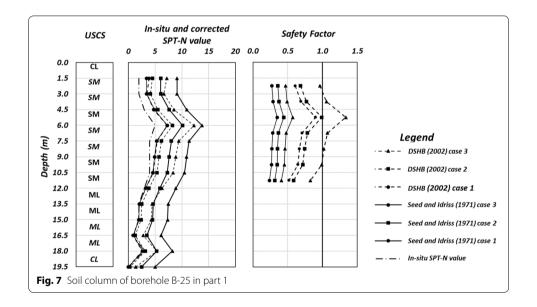
safety values are smaller for case 1 rather than case 2, and for case 2 rather than case 3 due to increase in the percent of fines content. Moreover, there is a notable difference in calculated factor of safety values through two methods, so that the obtained values by Seed and Idriss [1] method are smaller than those by DSHB [8] method in all the depths for three cases.
