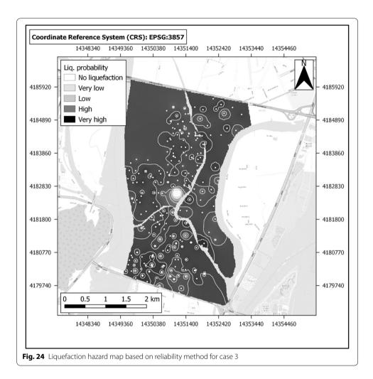
case of fines content through this approach. In contrast, the reliability approach showed less sensitivity (about 5%) to different percentages of fines content. The number of sites predicted to be liquefied by reliability approach are higher comparing to the deterministic approaches as well as the liquefaction severity.
