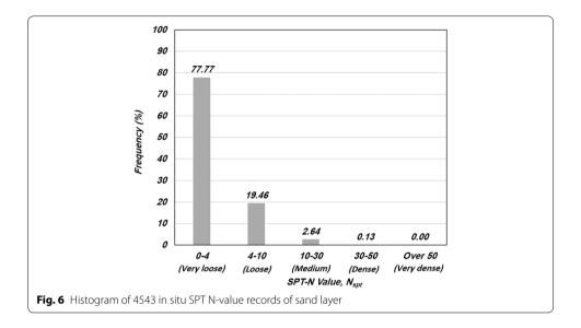
[18] and the histogram of them is shown in Fig. 6. This figure shows that over 75% of the soil layers in this area are lied in the range of very loose.
