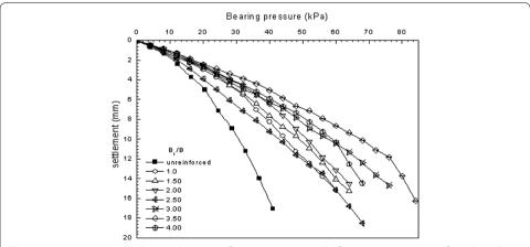
**Fig. 9** Bearing pressure-settlement behavior of 75 mm square model footing on geojute reinforced sand (reinforcement depth ' $D_r$ ' = 0.50B)
