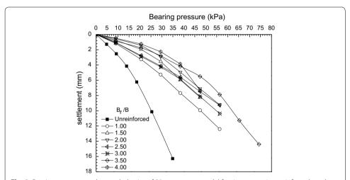
**Fig. 8** Bearing pressure-settlement behavior of 50 mm square model footing on geojute reinforced sand (reinforcement depth 'D $_{\rm r}$ ' = 0.50B)
