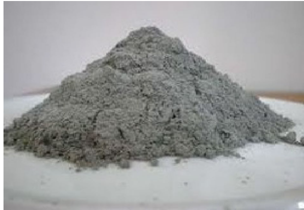
Fig. 2 Kakatiya thermal power station (KTPS) bottom ash
