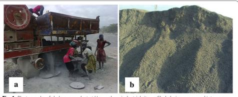
**Fig. 1** Photographs of shale quarry dust at Umuoghara industrial sites. **a** Shale being processed into aggregates with its dust. **b** Part of shale quarry dust used for the study
