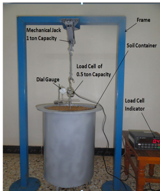
Fig. 9 Model pile pullout test system during testing
