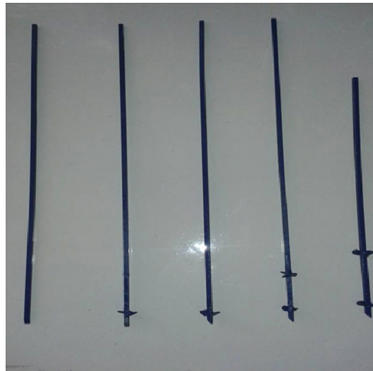
Fig. 1 Different types of helical piles used in the models
