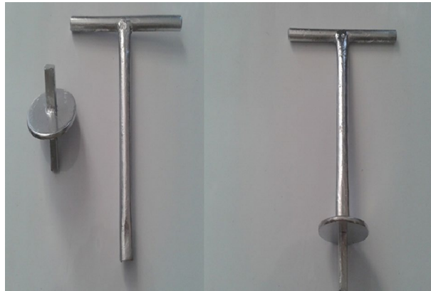
Fig. 6 Tools of helical pile installation in the soil
