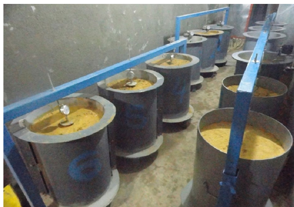
Fig. 7 Manufactured frames of uplift movement measurement of helical piles
