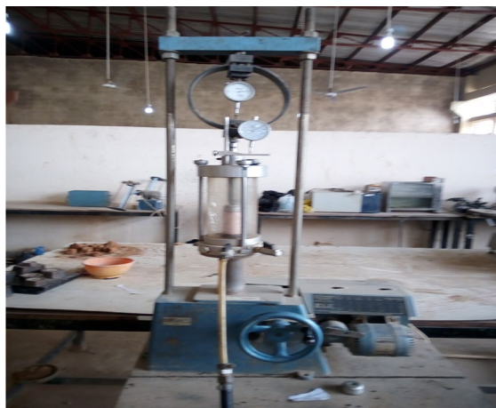
Fig. 3 Triaxial testing setup for unconfined compression test
