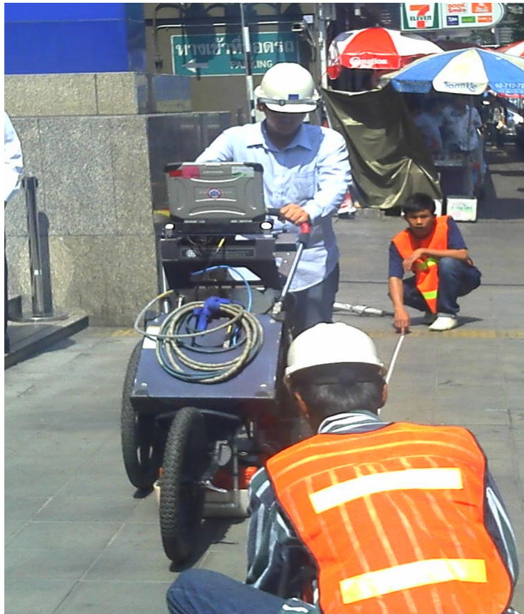
Fig. 2 GPR instruments and the survey cart used during the GPR data collection in the Bangkok area
